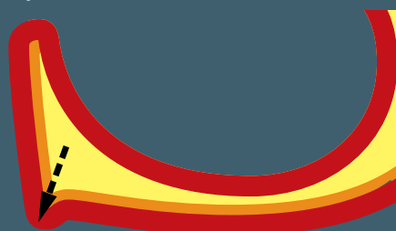
Spread: Lighter foreground extends over dark colour
